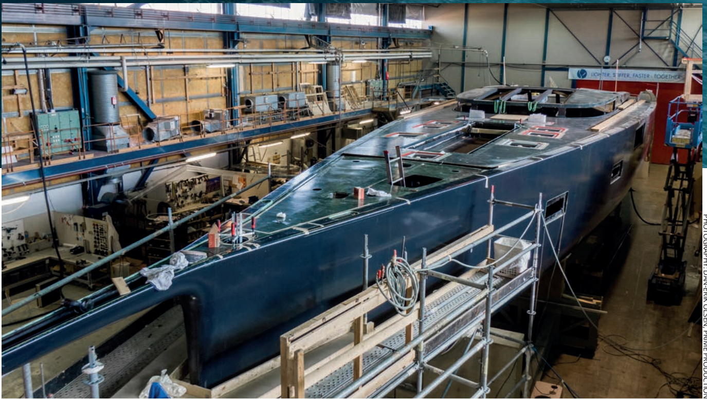
The hull and deck have been joined and fitting out is under way. Note the elegantly shaped, fully integrated bowsprit
