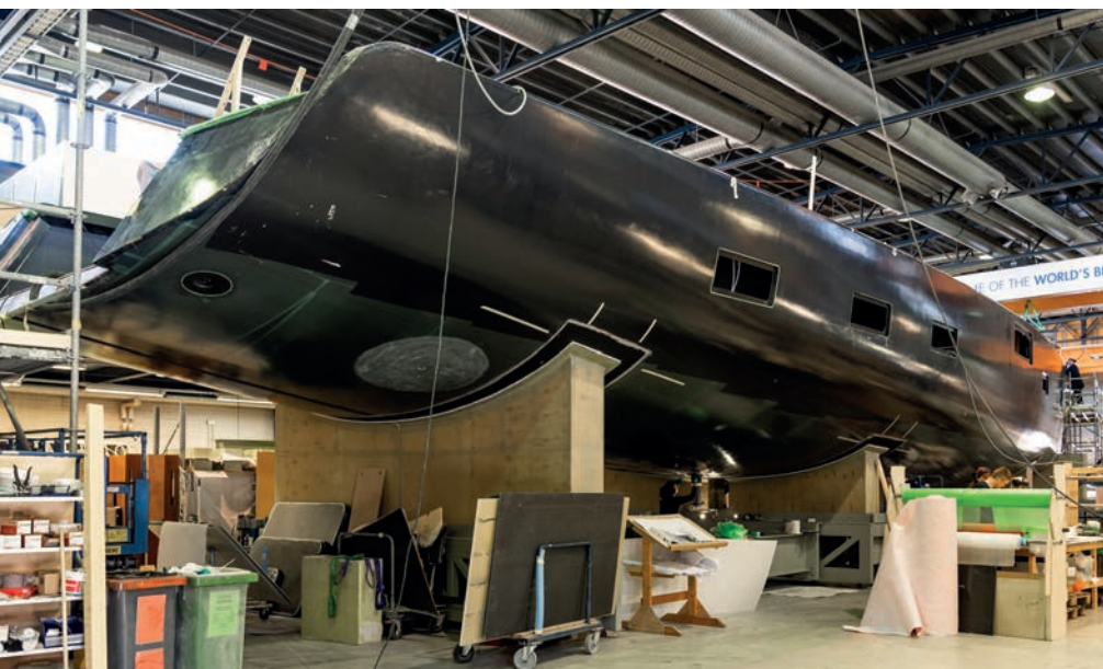
Broad aft quarters above the waterline add form stability when the yacht heels
