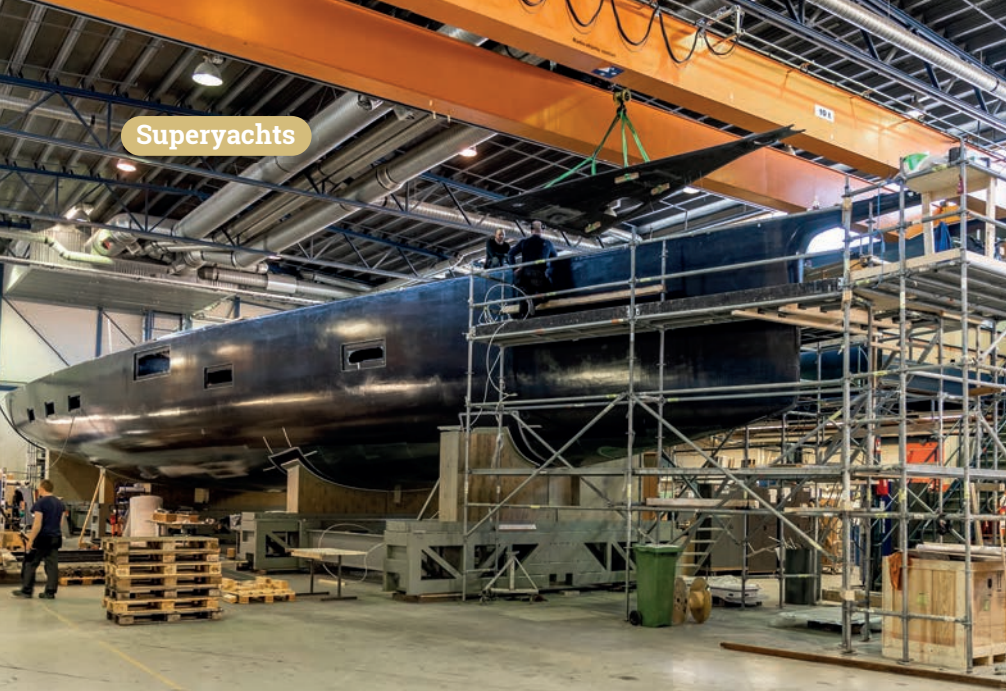
The hull shape has some modest rocker to improve motion comfort at sea
